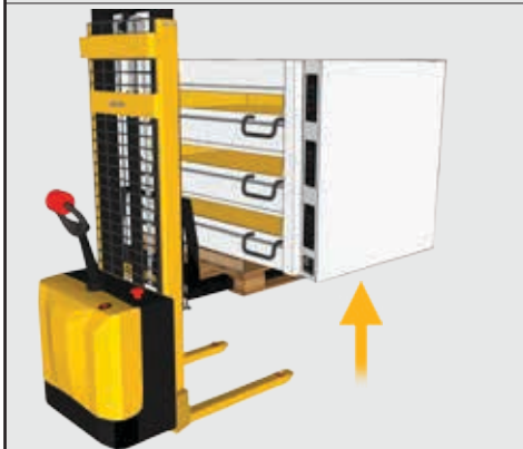
20. Carefully lift the oven using a pallet truck, forklift or Genie lift, depending upon the weight of the oven. (Continue at step 26)
