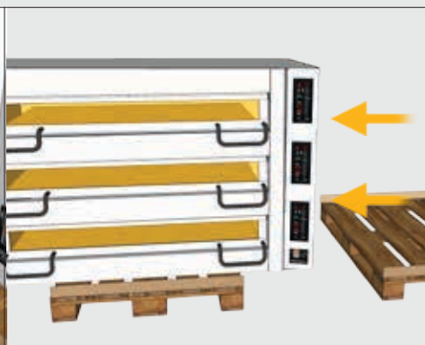
19. Push and center steady the oven over the biggest pallet and remove the other(s) pallet(s)
