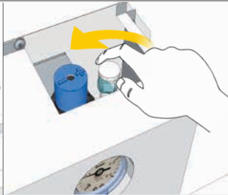
5. Turn ON the water and let water flow through the valve and then close the Air Relief Valve
